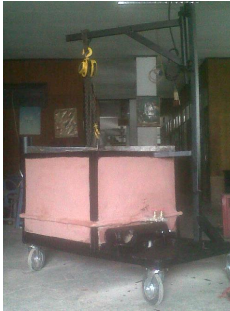
Gambar 3. Tungku Pack Carburizing Mobile
