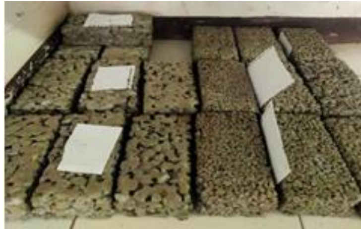
Gambar 4. Perawatan Benda Uji Paving Block Berongga
